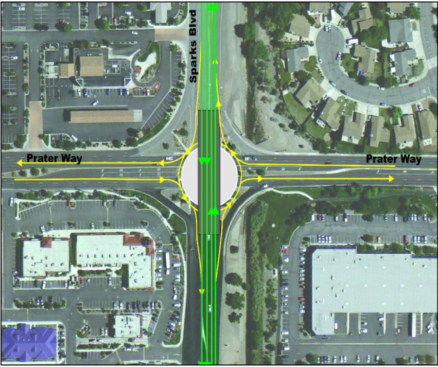
Figure B-5. Fly Over With Roundabout
