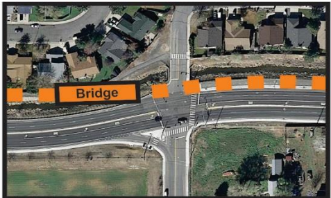
Construct ped/bike bridge creating a smooth transition for the path across the Truckee Drain.
