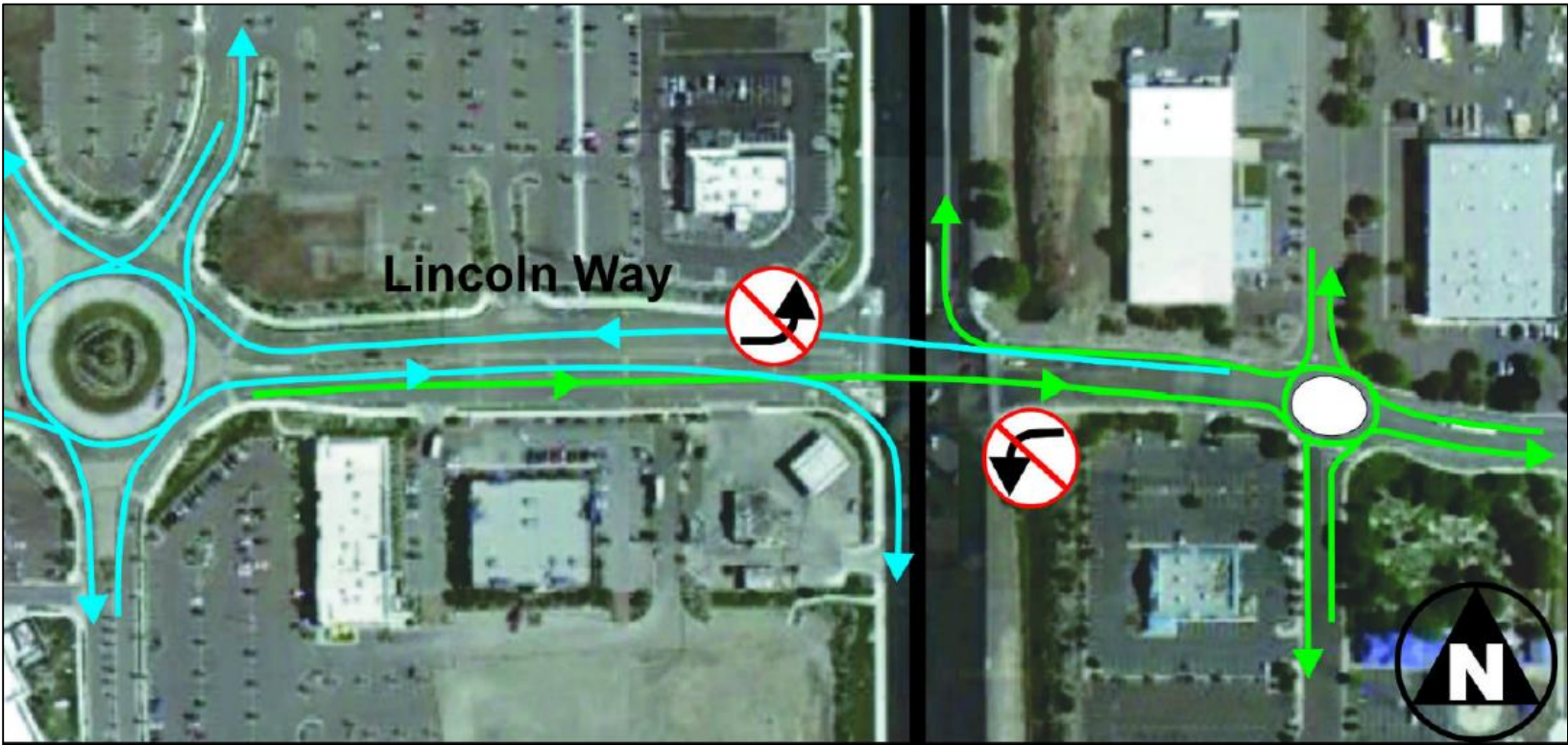
Figure B-11. Bowtie Intersection Concept at Sparks Blvd/Lincoln Way
