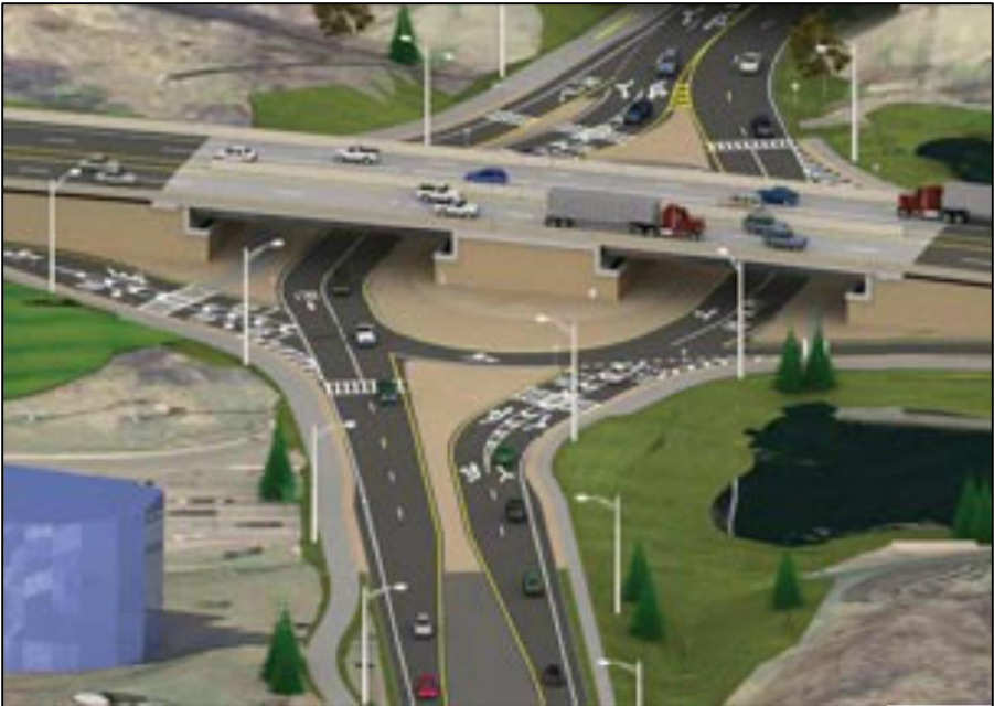
Figure B-6. Fly Over With Roundabout Underneath
