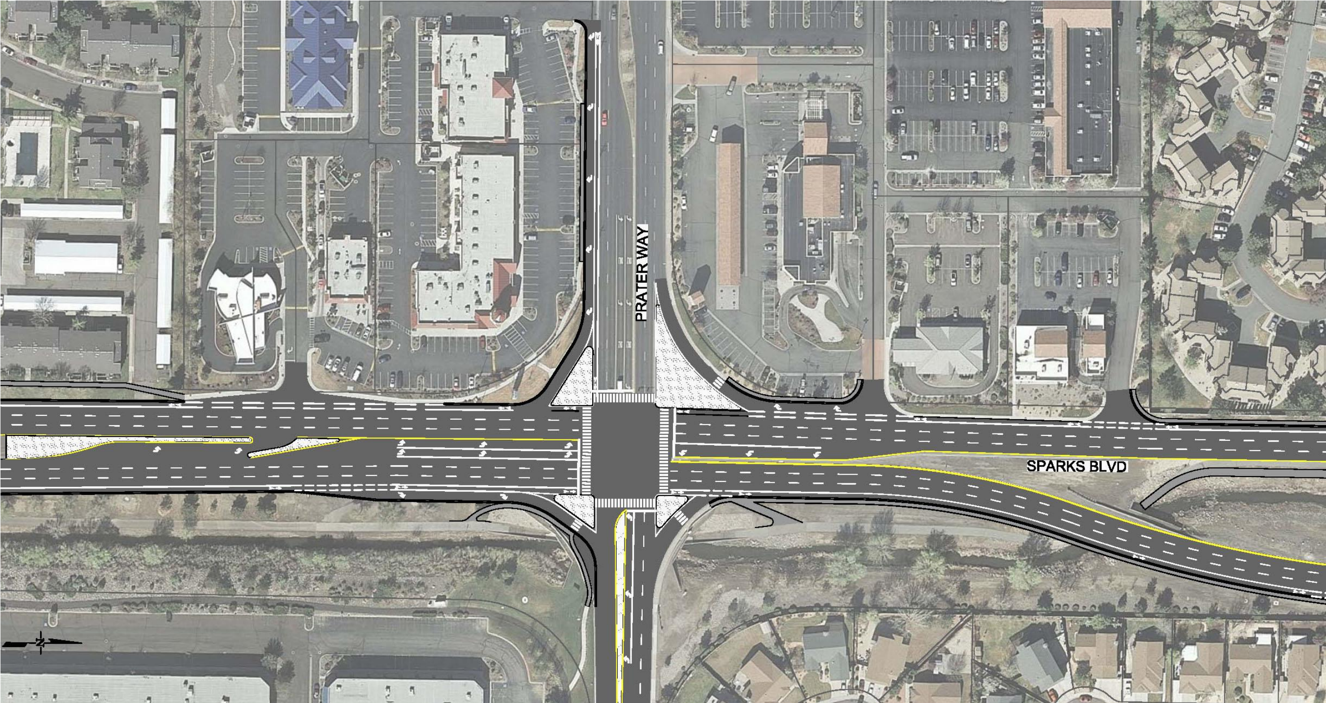
Figure 11-23. Ultimate Configuration at Sparks Boulevard/Prater Way
